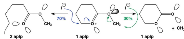
Fig. 16 Reaction of alkoxy-carbenium ion with iodide nucleophile.
