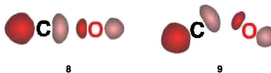
Fig. 8 Idealized \sigma^* C–O (left) and \tau^* C–O orbitals (right).
